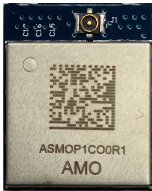
Figure 1. UWB SR040 Module with RF connector. (Top View)
